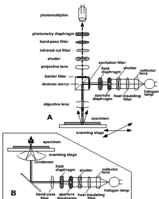
A second halogen lamp and a band-pass filter of various wavelengths in the visible region are mounted under the scanning stage. Thus, slices stained for histochemical or enzyme-labeled immunohistochemical analysis as well as films such as autoradiographs, can be analyzed quantitatively.
