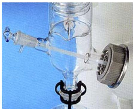
quickly by just turning the flask release nut. Vertical condenser (Glassware B&C) function to prevent liquid from stagnating. (patent pending) New condenser tubes (type A&B) designed to increase rapidity of cooling capacity.(Surface area is 20% larger than previous model.)
