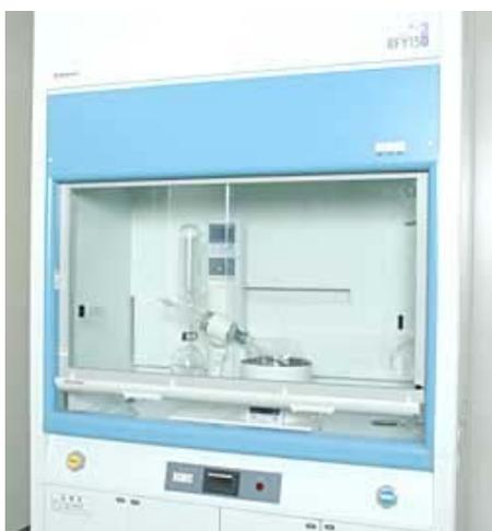
The rotary evaporator is compact, which can be neatly installed in a fume hood. Despite its depth of 400 mm, the vertical condenser (Glassware B/C) does not take up space.
