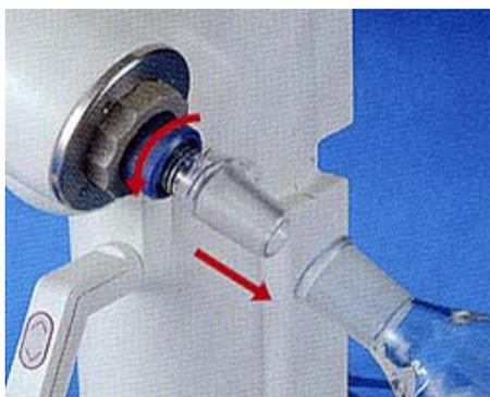
The evaporating flask can be released easily and quickly by just turning the flask release nut. vertical condenser (Glassware B/C) does not take up space.
