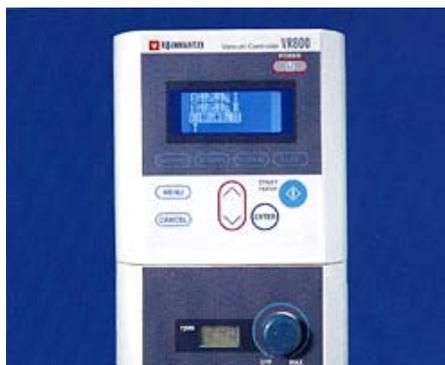
The evaporator's motor speed(rpm), vacuum(degrees) and vapor temperature can be digitally set and displayed. Experimental conditions and steps during a reaction can be saved and repeated in future. Display language can be chose either Japanese or English.(Only the rpm of the motor can be digitally displayed in model RE301.)
